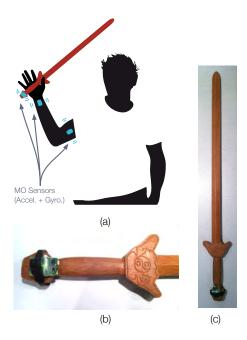
Figure 5.1: *Jian* sword Equipped with MO sensors, and disposition of other inertial sensors
