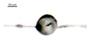
**Figure 5.3** – A bundle made from electrospinned block copolymer PVDF-HFP fibres (left) can be coiled within a silicone oil droplet (right). The nature and heterogeneity of the fibre bundle makes observation difficult.
