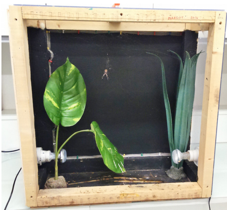
Figure 2.5 – Spider housing. It is 80 \times 80 \times 30 cm and consists of PMMA windows, wooden panels, artificial plants and warming lamps.
