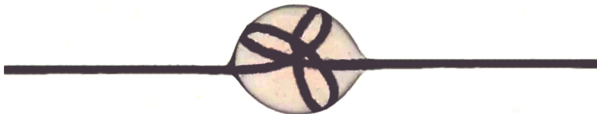
Figure 5.10 – A 2.7 mm silicone oil droplet coils a 140 \mu\text{m} polymeric fibre. A dense environment (water) is an effective way of upscaling the coilable fibre systems by use of Archimede’s forces. Source: Paul Grandgeorge.
