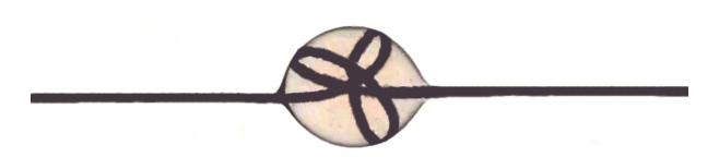
**Figure 5.10** – A 2.7 mm silicone oil droplet coils a 140  $\mu$ m polymeric fibre. A dense environment (water) is an effective way of upscaling the coilable fibre systems by use of Archimede's forces. Source: Paul Grandgeorge.
