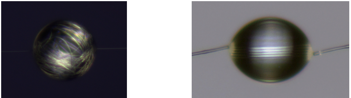
Figure 4.10 – Polarized light reveals the different morphologies of coiling in the TPU fibre/silicone oil droplet system: disordered (left) or ordered (right). The dark background is due to the polarizing technique.
