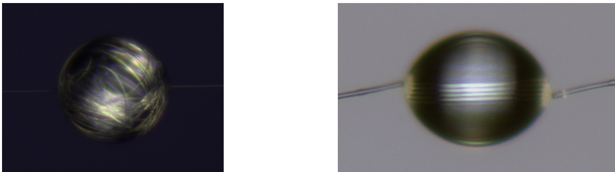
Figure 4.10 – Polarized light reveals the different morphologies of coiling in the TPU fibre/silicone oil droplet system: disordered (left) or ordered (right). The dark background is due to the polarizing technique.
