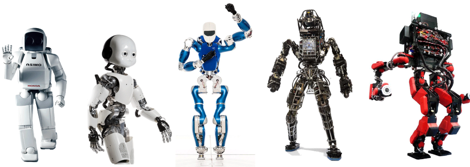
Figure 1.4.: Humanoid robots and their various shape and applications. From left to right — Asimo (home assistant, Honda, 2004), iCub (cognitive studies, RobotCub & IIT, 2004), TORO (interaction with the environment, DLR, 2013), Atlas (disaster response, Boston Dynamics, ca. 2013), SCHAFT (disaster response, SCHAFT, ca. 2013).
