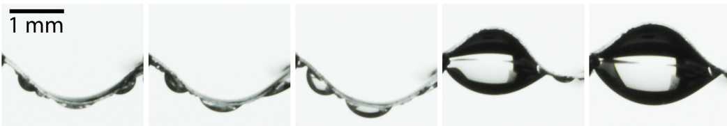
FIG. 3.10 - Condensation-induced snapping. The experiment approximately lasts three minutes.
