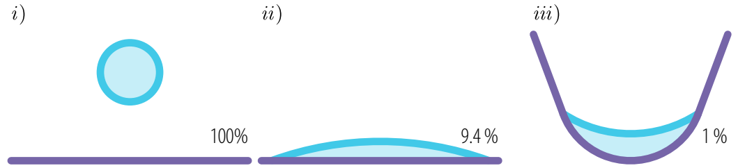
FIG. 3.1 - A 2D energetical view on elastocapillarity. We start by considering a rigid ground (reference energy level). i) A droplet is introduced and adopts a circular shape. The energy of this configuration is E_0 = 2\pi R\gamma_{\ell v} . ii) If the drop touches the substrate, the total energy is lowered to 9.4% E_0 for the parameters used in the model (see text). Note that the exposed free surface is extended, but that the energy gained by wetting the surface largely compensates for this additional cost. If the wet footprint was larger, the cap would have a too large area and the energy would be higher. If the footprint was smaller, the energy gain by wetting would not be maximal. The better trade-off therefore corresponds to this situation where the contact angle of 20^\circ is given by Young-Dupr e wetting relation. iii) If the surface is made flexible, the elastic energy cost of bending is again largely recovered by the less exposed free surface allowed by this folded configuration. The energy is here 1% E_0 .
