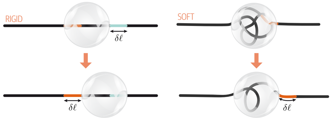
FIG. 4.5 - Why is there a tension? Left: a drop can slide over a rigid fibre at no energetical cost, \delta E = 0 . The tension in the fibre is therefore zero, as expected from the cancelling of the facing meniscus forces. Right: if some slack fibre is spooled inside the droplet, an energy is required to pull out the fibre from the droplet: the fibre is under tension.
