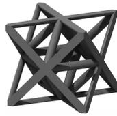
Figure 2.4: The octet truss unit-cell, proposed by [Fuller, 1961]
