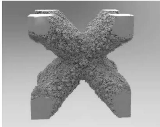
Figure 2.7: 3D reconstruction of one lattice unit-cell (3 mm side length, 1 mm strut diameter) characterised through  $\mu$ -CT
