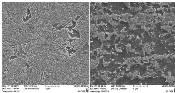
Figure 2.22: SEM micrographs of DP1180 base metal (left) and heat affected zone (right) after welding using 4kW Nd:YAG laser at 3.5m/min, adapted from ArcelorMittal internal report *in* [Shome and Tumuluru, 2015]. Bright grey denotes martensite, dark grey is ferrite.
