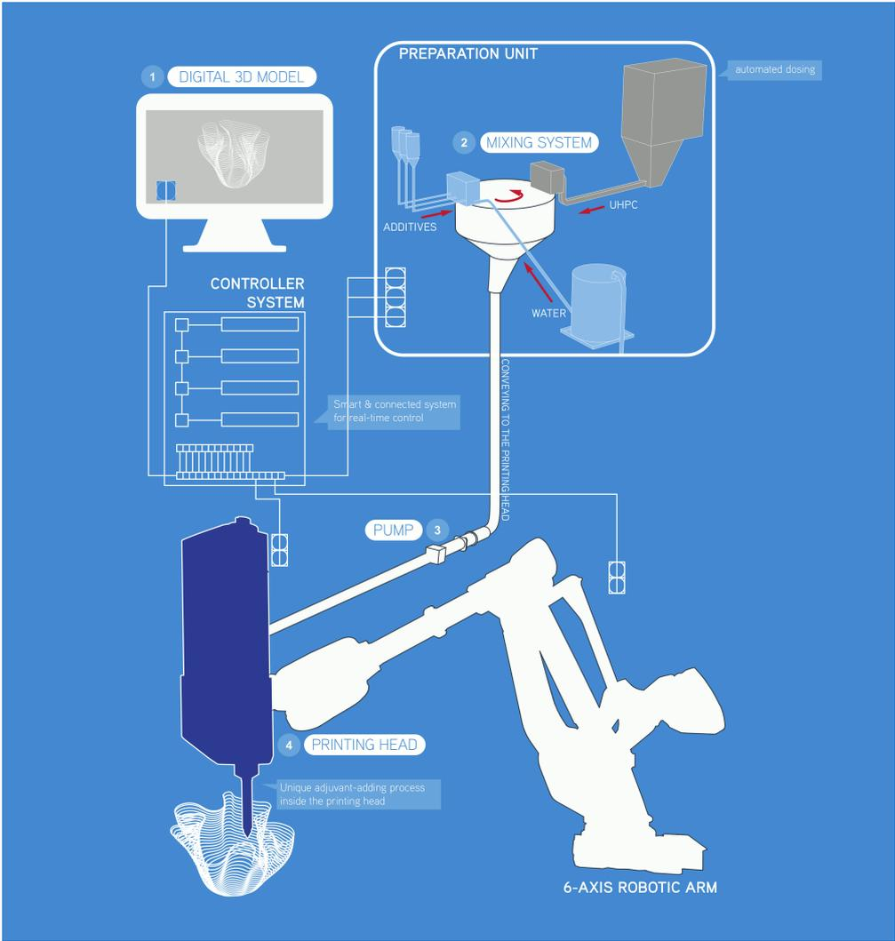
Figure 3.4: Workflow of the large-scale concrete additive manufacturing
