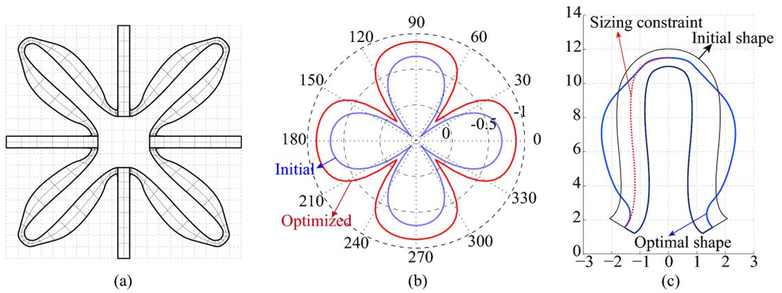
Figure 2.18: Full model of the optimised design (a); polar plot of the effective Poisson ratio for the optimised design (b); comparison between the size bounding polynomials, the initial and optimised designs (c)
