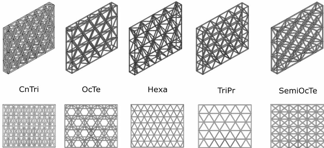
Figure 3.13: Various grid topologies for space truss tessellation
