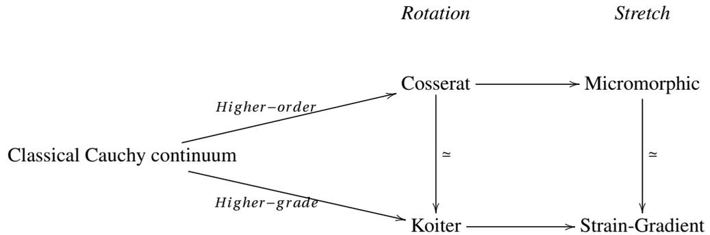
Table 2.2: Extensions of a Cauchy continuum. From the left to the right, *rotation* then *stretch* are added to the kinematics. For higher-order continua these extensions are independent DOF, for higher-grade continua they are controlled by higher-order gradients of the displacement field.
