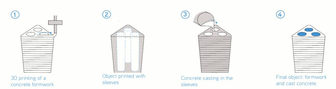
Figure 3.5: Schematic view of the concrete formwork 3D printing process
