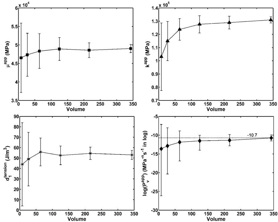
Figure 1.11: The mean values for the apparent properties with increasing volume size. The error bars correspond to plus and minus 2 standard deviations
