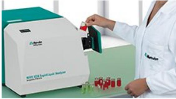
(a) Appareil *Near InfraRed Spectroscopy* (NIRS) de laboratoire [53]
