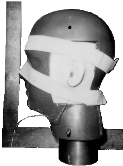
b. BAMAR head with pinna molds attached.
