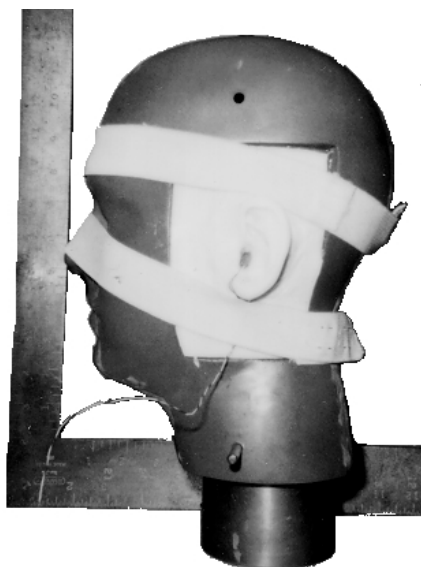
b. BAMAR head with pinna molds attached.
