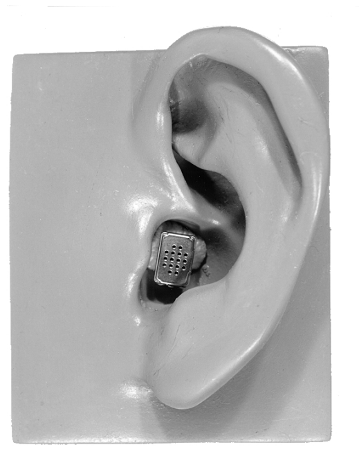
a. Pinna mold with microphone in place.
