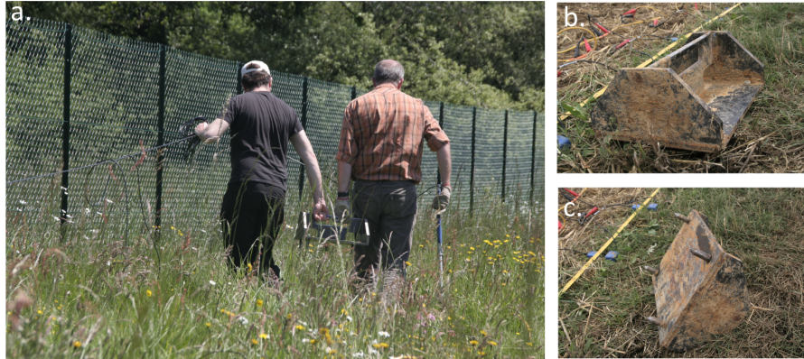
Figure 3.4: (a) Christian and I carrying the S-source. (b,c) Top and bottom view of the frame. As noticed in the Merlimont experiment, this source is efficient only if one stands on the frame to increase its coupling with the ground while a second operator is trying to hit it as horizontally as possible, which is quite unsafe. Modified after Pasquet (2014).
