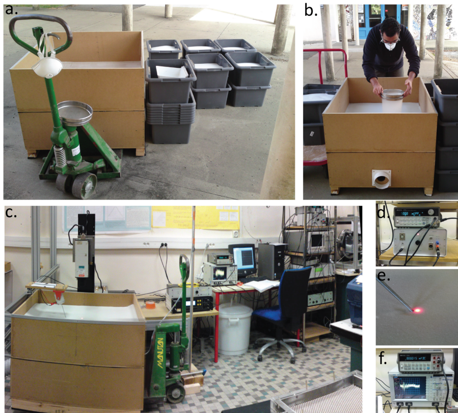
Figure 1.5: Physical model construction and set-up for granular media: (a) we used calibrated glass beads (a lot!) or sands of various diameter sizes and distributions; (b) the material was poured or sieved, vibrated or not, depending on both its type and anticipated mechanical properties of the model (the process is detailed in the following section); (c) the global view of the set-up shows typical items for the acquisition (quite similar to those presented earlier...), except for the source which consists in a metal stick attached to a low-frequency shaker (a great variety of source, shakers, orientations, coupling etc had to be tested (Jacob et al., 2008; Dhemaied, 2011) before obtaining satisfying and reproducible results (Bodet et al., 2014b)). (d, e, f) detailed views of the amplifier used for the force source signal, the stick and scattered laser spot (another issue of the process to be discussed) and the oscilloscope stacking the acquisitions...
