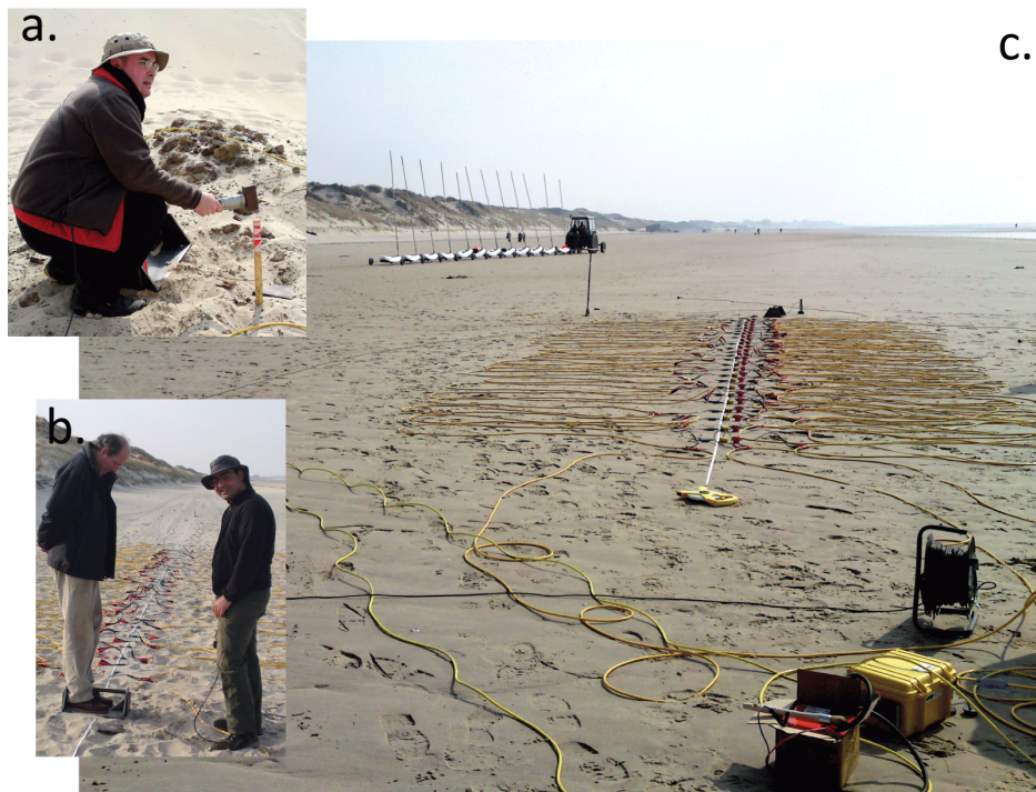
Figure 3.1: Mimicking Bachrach and Nur (1998); Bachrach et al. (1998) and West and Menke (2000) experiments in Merlimont (Pas-de Calais, France). (a) Fayçal Rejiba hitting the sand as vertically as possible to provide seismograms for P-wave refraction. (b) Christian Camerlynck standing on our S-source to increase its coupling with the ground while Amine Dhemaied is getting ready to hit it as horizontally as possible to provide seismograms for SH-wave refraction. (c) Global view of the 3-component set-up dimensioned by Mickael Duranteau during his Master internship in 2010 (Duranteau, 2010).
