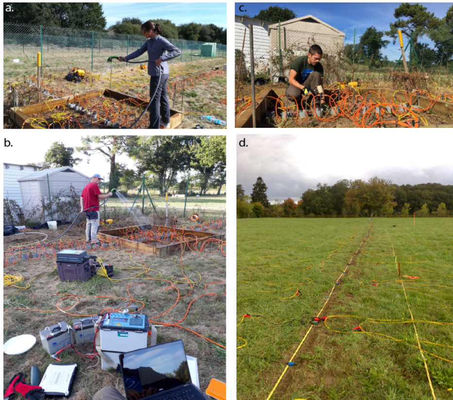
Figure 3.23: (a, b, c) Lara Blazevic (PhD thesis, ITN ENIGMA, Sorbonne Université 2017-2020), Laurent Longuevergne and Sylvain Pasquet (Post-Doc OZCAR 2018-2020) performing an infiltration experiment monitored by time-lapse seismic and electrical methods as well as underground TDR probes. (d) Experimental set-up designed to perform comparisons between 3-component seismic acquisition with Fiber Optic Distributed Acoustic Sensing, the fiber-optic cable being buried in a trench below the geophones (CRITEX/H+ Workshop in Poitiers, Oct. 2015).
