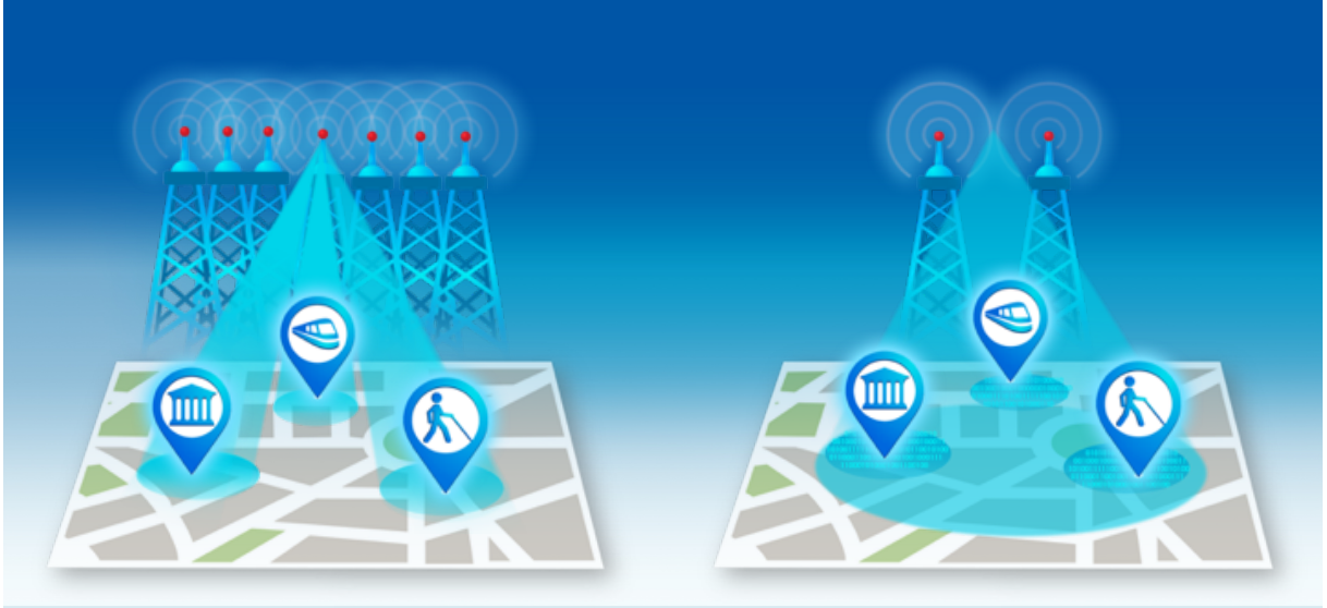
Figure 4.1: Example of geocasting with Beamforming (on the left) and with Spatial Data Focusing (on the right).
